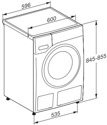
W1 drawing, facia 5 degree, mesures in mm
